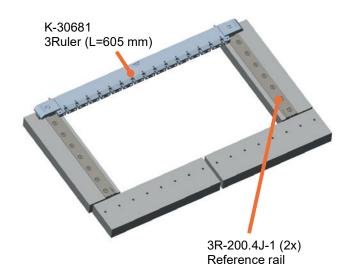
Machine table without tooling Working area:
