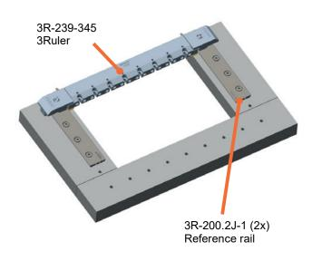
Machine table without tooling Working area:
