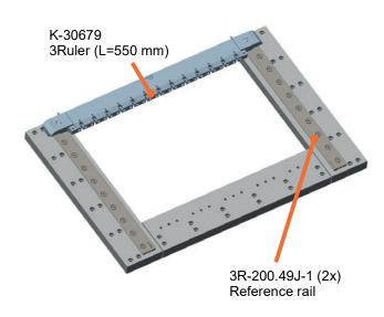
Machine table without tooling Working area:
