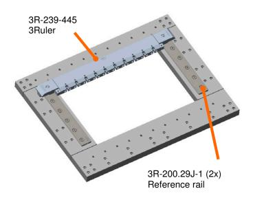
Machine table without tooling Working area:
