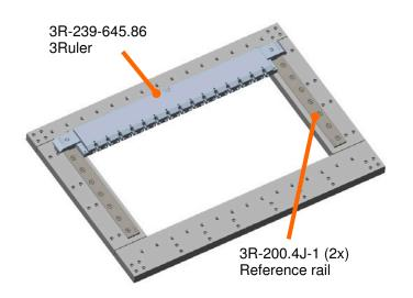
Machine table without tooling Working area:
