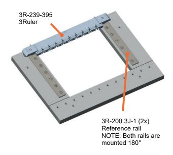
Machine table without tooling Working area:
