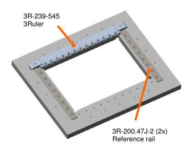
Machine table without tooling Working area:
