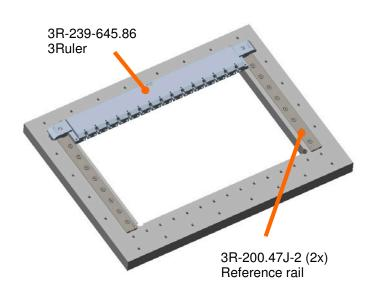
Machine table without tooling Working area:
