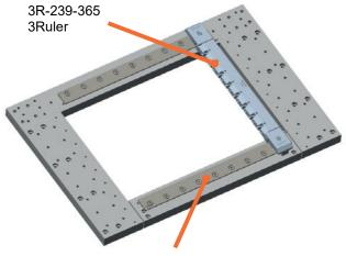
3R-200.44J-1 (2x) NOTE: Both rails are mounted 180°. Reference rail may alone or together with 3R-200.4J-1 support products other than 3Ruler.
