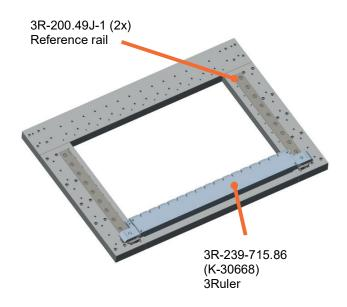
Machine table without tooling Working area:
