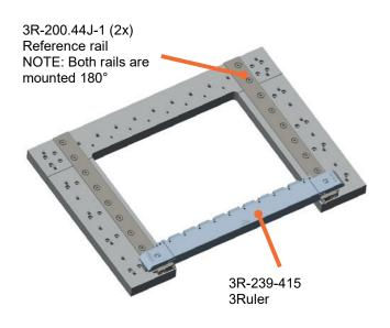
Machine table without tooling Working area:
