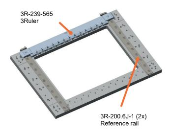
Machine table without tooling Working area:
