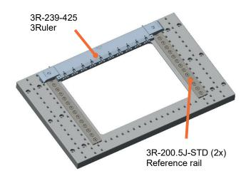
Machine table without tooling Working area:
