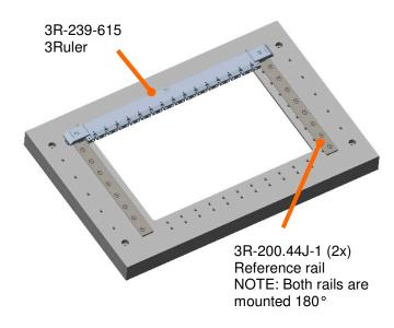
Machine table without tooling Working area:
