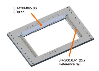
Machine table without tooling Working area:
