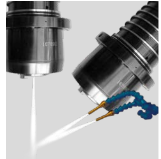
Air through spindle/spindle slots
