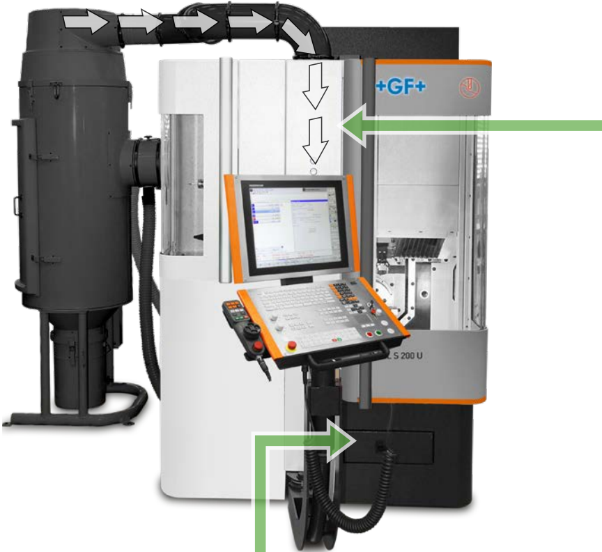
Supply air for dust extraction
